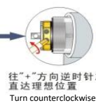
c. 调下限位调上旋钮 Adjust the lower limit and th upper knob.
